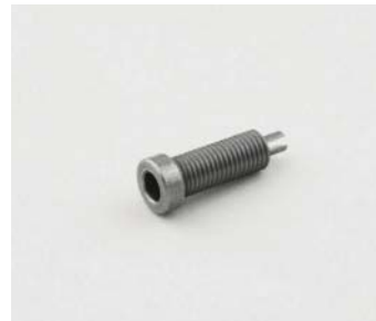
BU V2A 4000 Panel mount socket 4 mm Ø with solder connection and external thread M 6x0.75 from V2A steel.
