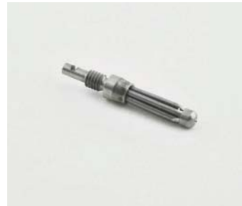
S V2A 4000 Bundle contact plug 4 mm Ø with protective cap and M 4 thread with solder connection, from V2A steel.
