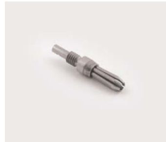
N V2A 4000 Bundle contact plug 4 mm Ø with M 4 thread and solder connection, from V2A steel.
